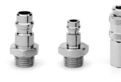
The Series 5000L and 5000LT couplings have been designed to connect tubes for water, air or oil, used within plastic injection and die casting moulds. The Series 5000L and 5000LT couplings provide a quick connection and disconnection method for the replacement of heating and conditioning tubes directed towards the mould, as well as tubes coming from water collectors or sources.
